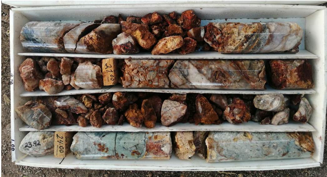
Figure 10-1: Typical drill hole recovery and RQD (RDO-20-090)
