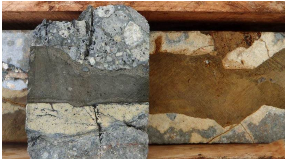
Figure 7-10: Late-stage pyrite-marcasite mineralization and its oxidized equivalent
