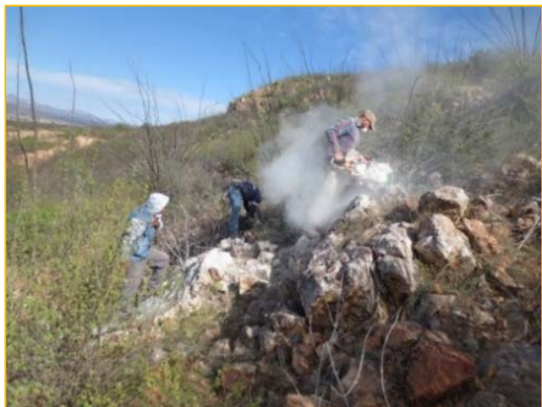
Sawing channel samples
