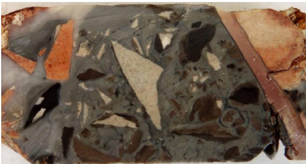
FIGURE 7-8: SEVERAL STAGES OF LATE SILICA CEMENTING BRECCIAS
