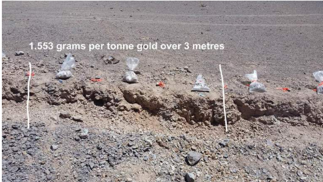
Figure 9.3 - Photograph of Trench SE 2012-02, note recessive nature of grey, sericitic alteration. Orange flagging represents metre marks.
